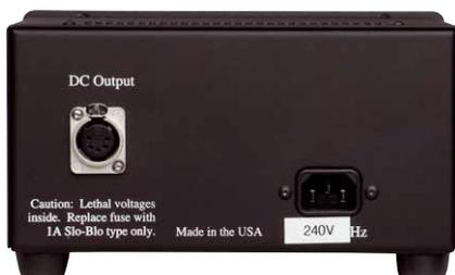
*The special sockets prevent incorrect connection of the power supply*
