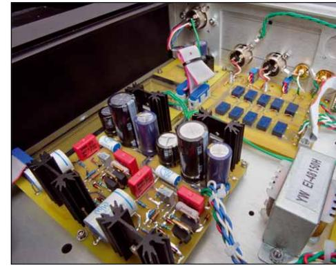
*Situated right in device, there is another power supply board for voltage regulation; behind it is a whole bank of relays to switch the gain stages*
